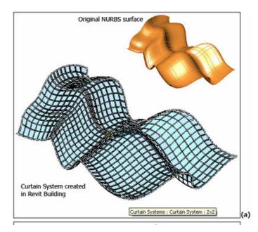
Now I generated this particular surface in Autodesk 3dsmax using a plane, with FFD box to deform it and then adding a mesh smooth. After taking it to revit the results I had trying to turn the surface to a curtain wall were undesirable.
