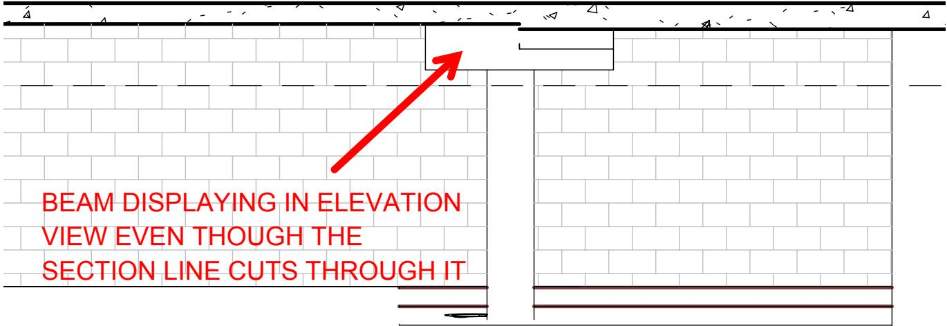
BEAM DISPLAYING IN ELEVATION
