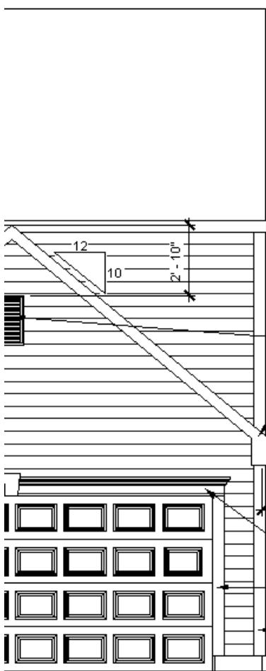
Building from the ground up, once the 2nd floor has been constructed 2nd floor window and plate heights are dimensioned from a 0'-0" 2nd floor reference. This is how I need the 2nd floor level heads to display in elevation views.
