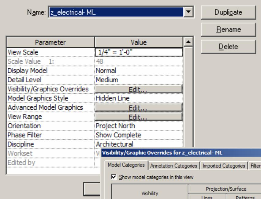
“View Template” used to convert a ceiling plan into a **LIGHTING + ELECTRICAL PLAN**.
