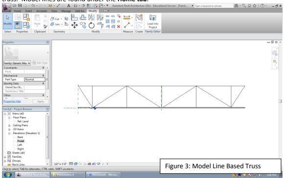
7. After finalizing the geometry of the truss, **trace the model lines** using structural members. This is accomplished by going to **Home Tab→ Component**. Note: When modeling the structural members, Revit automatically will adjust members to tolerances which will not show the member connecting to the truss.
