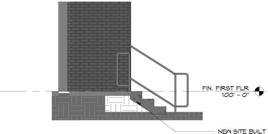
NEW SITE BUILT CONCRETE STAIRS. SAWCUT AND REMOVE EXISTING STAIRS THIS LOCATION.
