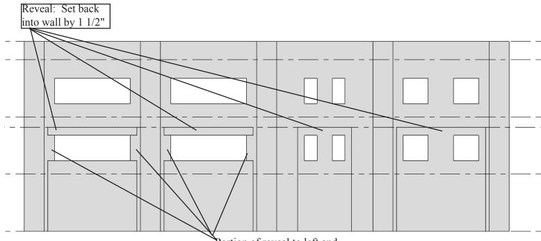
Portion of reveal to left and right of openings which is not "revealing" when openings are placed.
