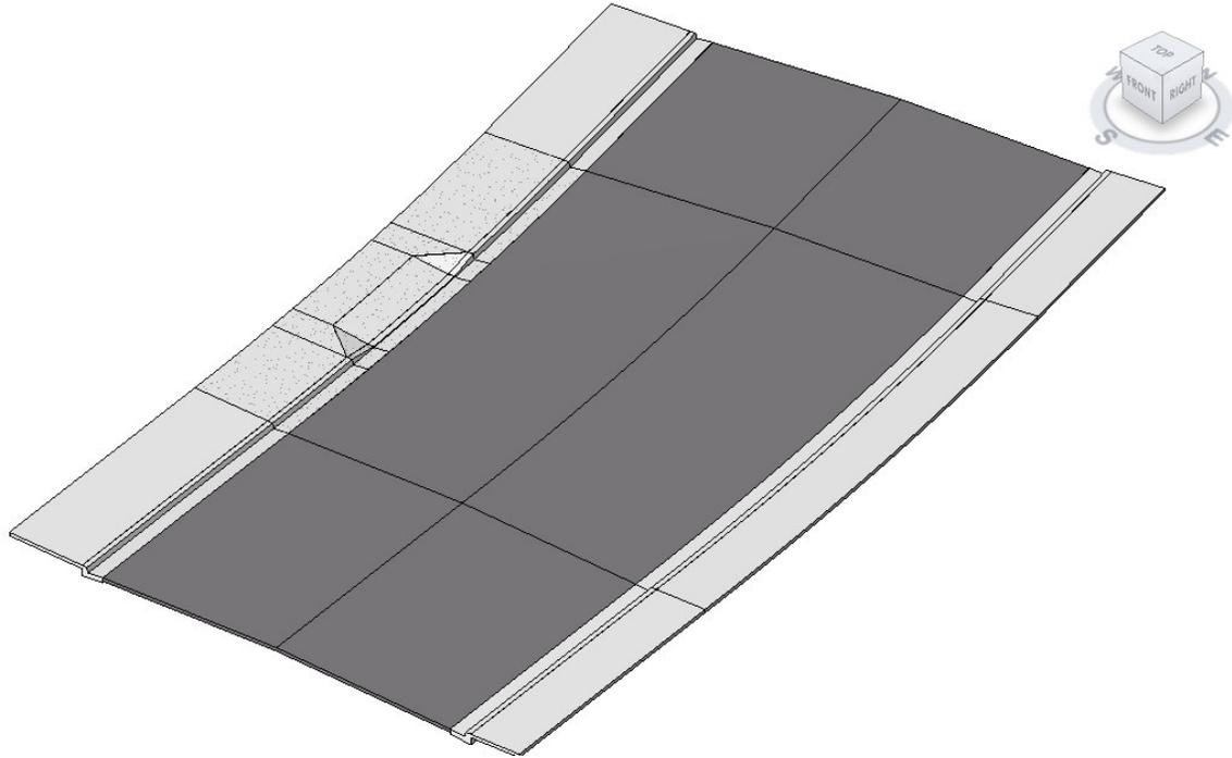
Then use the Solid Sweep Blend to create your path and cross sections and extrusions. The Solid Sweep Blend can only use one path at a time. The Solid Sweep Blend cannot use a straight portion of path and a curved portion of path at the same time. This model was created using centerline. Numerous sections will be needed to establish your model correctly. Adjust the elevation of each section height at each end of the path. Use the framing views to keep your sections square to the center line.
